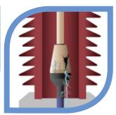
3. Undetected PD causes flashover and sudden failure
