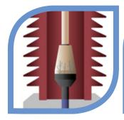
PD starts to erode insulation
