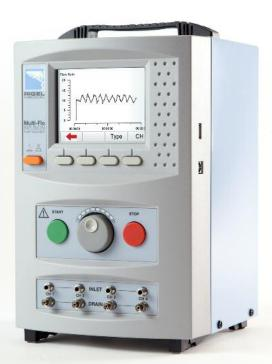
A remote (PC) control interface is available via Rigel's test solution software, Med-eBase, allowing complete control of the Multi-Flo's features from the comfort of a PC. Requiring just a single USB connection per Multi-Flo, the total number of pumps under simultaneous test is limited only by the number of USB ports available. Perfect for high volume test environments.
