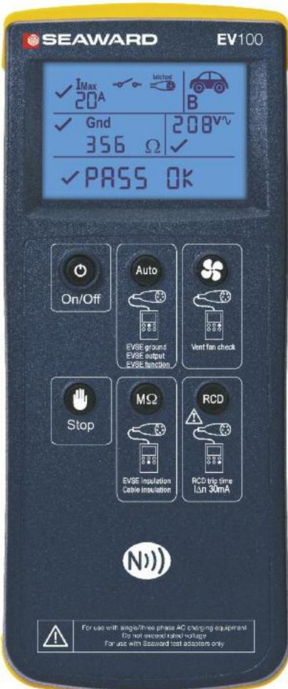
Whilst a basic set of measurements is clearly shown on the EV100 display, a much more comprehensive set of diagnostic data is stored in the EV100's internal memory.
