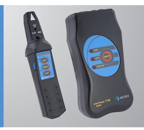
The MI 2093 Line Tracer is a universal instrument intended for tracing hidden conductive paths under plasters in walls, floors and ground or for determining one wire in a tuft of wires. Fuses or outlets belonging to a certain loop car be located as well. Line Tracer helps the operator to resolve hidden line problems easily (short circuits, interruptions, breakages).
