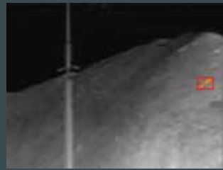
Smouldering detection (coal pile)
